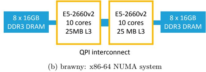
Figure 2: Demonstration platforms: (a) a wimpy smartphone system and (b) a brawny server system
